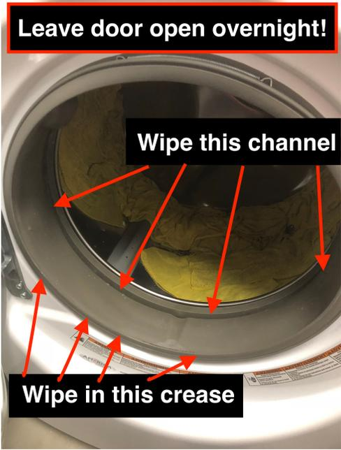
A photograph of the interior of a front-loading washing machine door. The door is open, showing the rubber boot. Red arrows point to specific areas: the top channel, the bottom crease, and the interior of the boot. Text boxes with red borders are overlaid on the image: "Leave door open overnight!" at the top, "Wipe this channel" in the middle, and "Wipe in this crease" at the bottom. |
